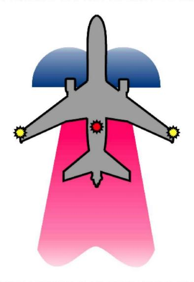
NEVER APPROACH OR WALK OR DRIVE BEHIND AN AIRCRAFT UNTIL THE ENGINES HAVE STOPPED AND THE ANTI-COLLISION LIGHTS ARE OFF
