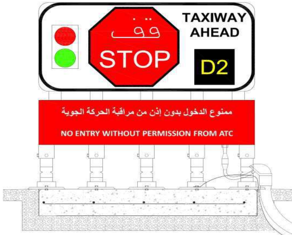
Figure 5-31. Road Holding Position Sign and Lights
