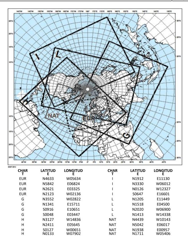
Figure A8-2. Fixed areas of coverage of WAFS forecasts in chart form —Polar stereographic projection (northern hemisphere)
