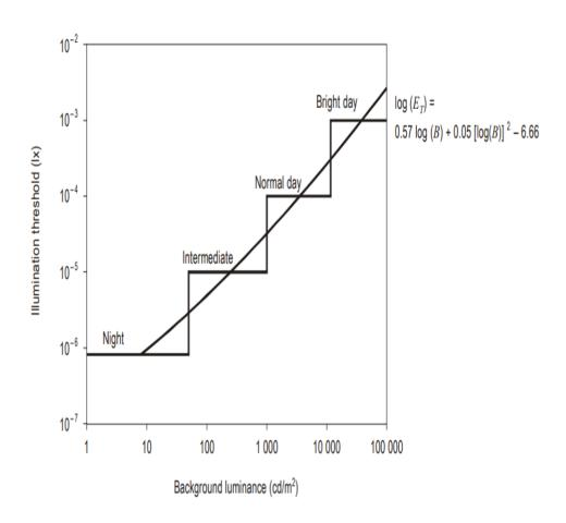
Figure D-1. Relationship between the illumination threshold  $E_T$  (lx)and background luminance B (cd/m²)
