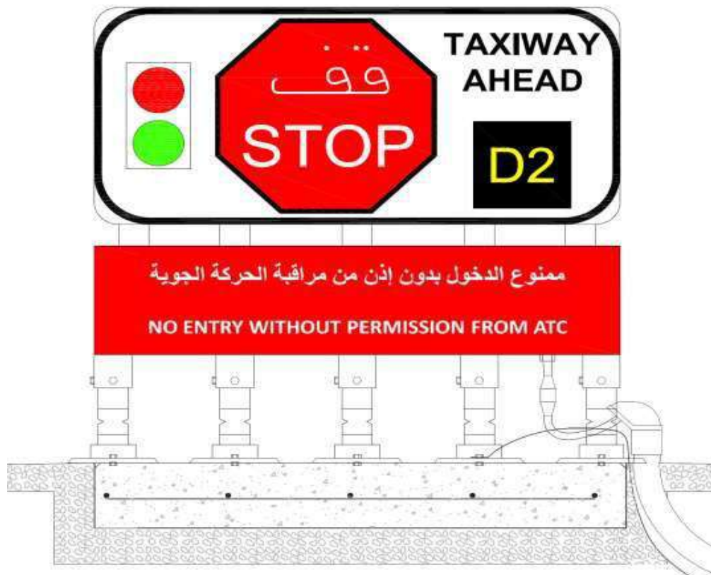
Figure 5-31. Road Holding Position Sign and Lights
