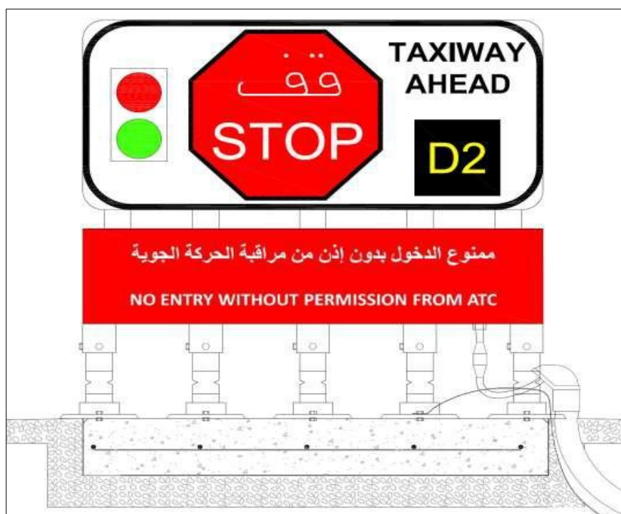
Figure 5-31. Road Holding Position Sign and Lights
