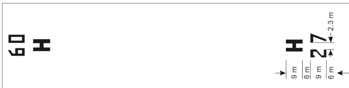
Figure 5-3. FATO designation marking and heliport identification marking for a runway-type FATO
